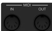
**MIDI Input and Output** - One 5-pin MIDI input port and one 5-pin MIDI output port for sending and receiving MIDI data between your computer and external MIDI devices.
