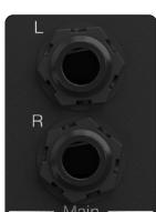
**Main Outputs (Ch 1 - 2, Left and Right)** - Use Main L and R to connect to your primary set of studio monitors.
