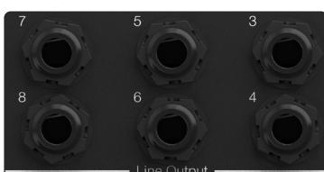
**Line Outputs (Ch 3 - 8)** - The Quantum LT 16 includes six TRS line outputs on 1/4-inch jacks for sending audio to line level devices. All LT 16 line outputs are DC-coupled for CV integration with CV-enabled equipment such as modular synths.
