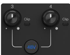
**Channel Gain Knob** - Use this knob to increase or decrease gain for the mic inputs on the back panel. The Quantum LT 4 has two gain knobs, controlling channels 3 and 4. The Quantum LT 2 has one channel gain knob which controls channel 2.
