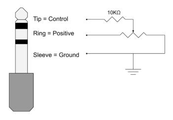
The following diagram shows how to create a cable to convert a volume pedal to an expression pedal.
