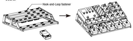
**NPB-L** : 320(L)x445(W)x90(H)mm ( For 10-12 pedals ) **NPB-M** : 243(L)x445(W)x90(H)mm ( For 8-10 pedals )
