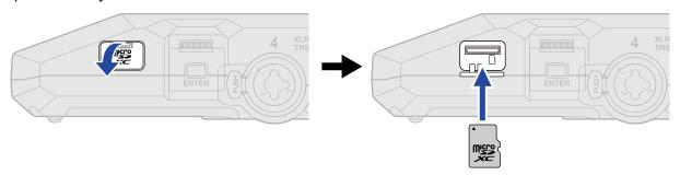
To remove a microSD card, push it further into the slot and then pull it out.
