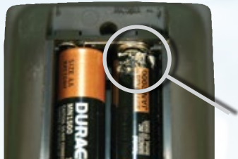
Corrosion you CAN see
