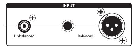
**Line-level Inputs.** The Eris Studio-Series monitors provide a choice of three line-level input types: balanced XLR, balanced ¼"TRS, and unbalanced RCA. Do not connect more than one source to your Eris studio monitors simultaneously.
