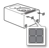
(4) Foam feet to be placed on the bottom of the speaker to improve isolation  $% \left( 1\right) =\left( 1\right) \left( 1$
