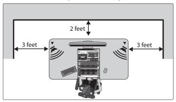
Just like it's not a good idea to set up your mix position in a corner, it's not a good idea to create a corner with your mix position. Make sure the distance from the speaker to the wall behind it is different than the distance from the side wall closest to it. For example, if your left speaker is one foot from the wall to its left, it shouldn't also be one foot from the wall behind it.
